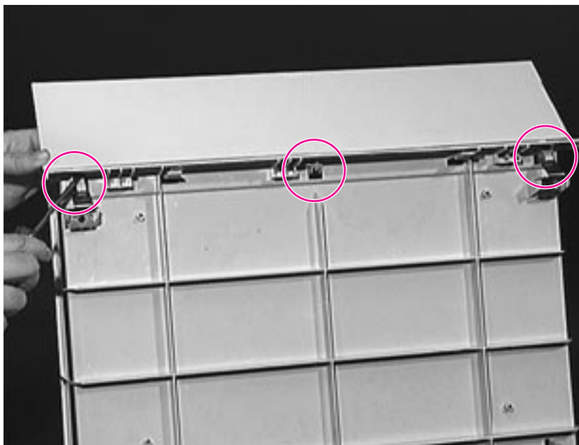
Figure 6-151 Front Door (Storage Area)
